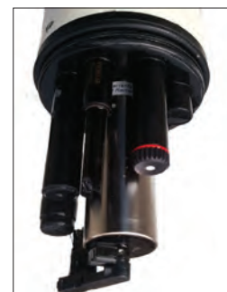
WQ-PAD platform, instrumentation and multi-parameter sonde
