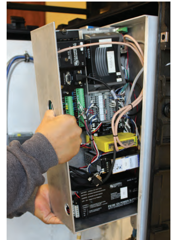
A portable, rugged, fully self-contained water quality station with easy access and instrument swap out capabilities.
