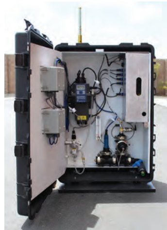
A portable, rugged, fully self-contained water quality station with easy access and instrument swap out capabilities.
